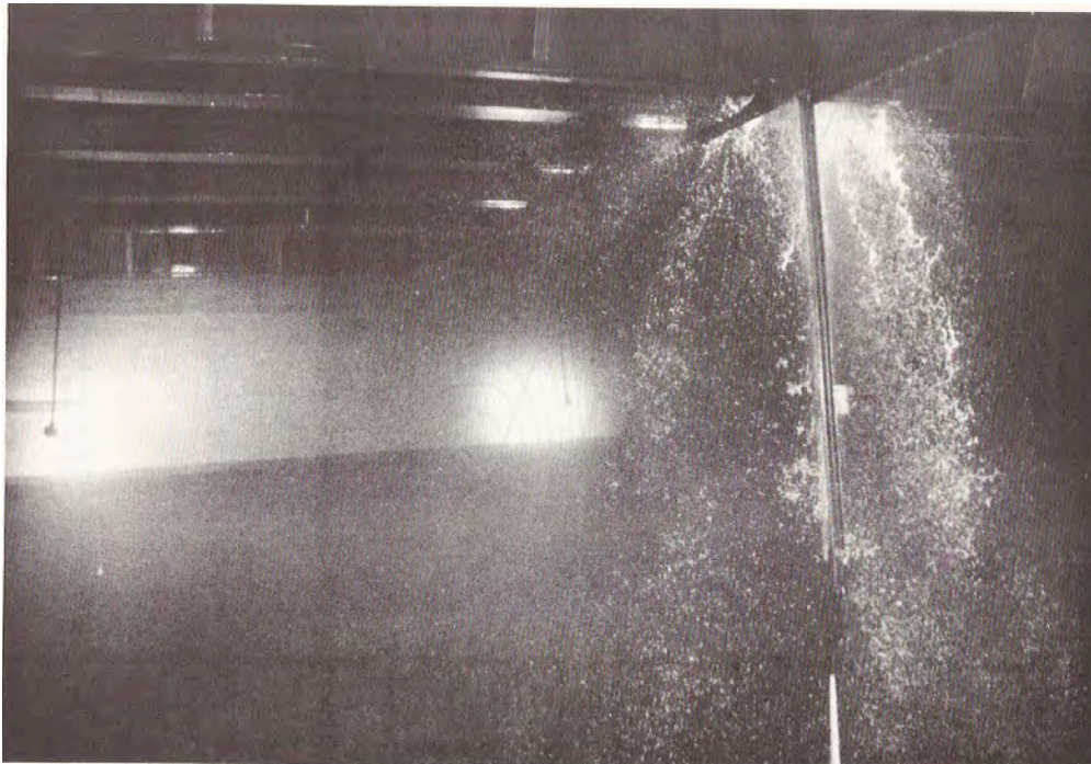
Figure 7.4: Example of flash photograph during washing triggered by occurrence of a spark
